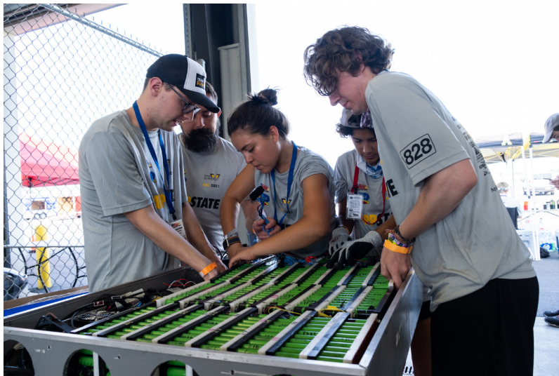
Figure 2. American Solar Challenge 2021, Solar Vehicle team working on battery pack before the race starts in Topeka, Kansas.
