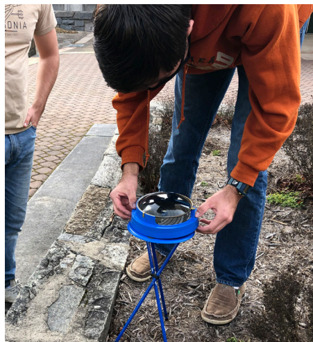
Figure 10. REI students placing the solar pathfinder due North to trace the shading on the dome.
